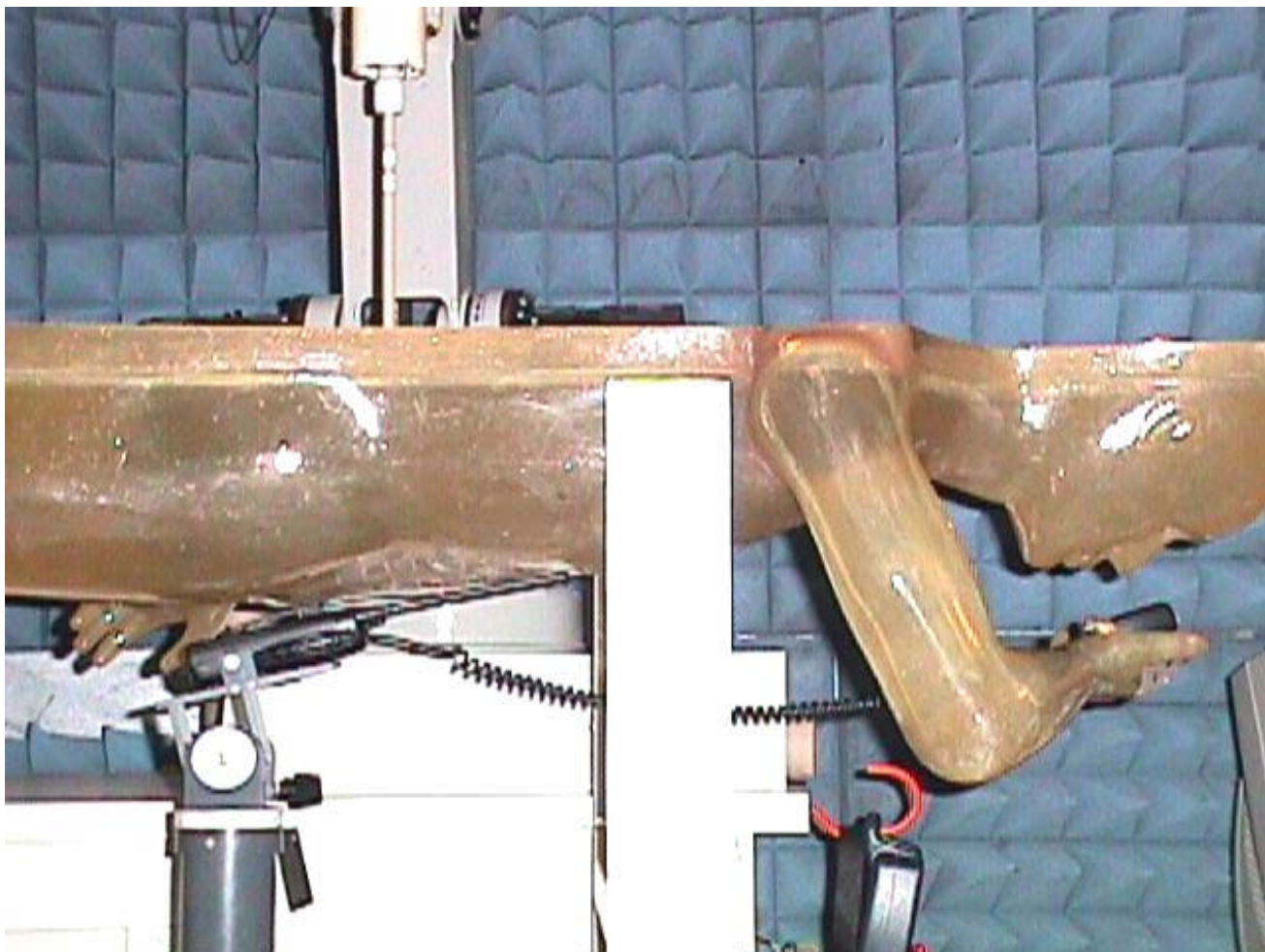
<Overview – Waist with normal belt clip and the antenna touching the phatom>
