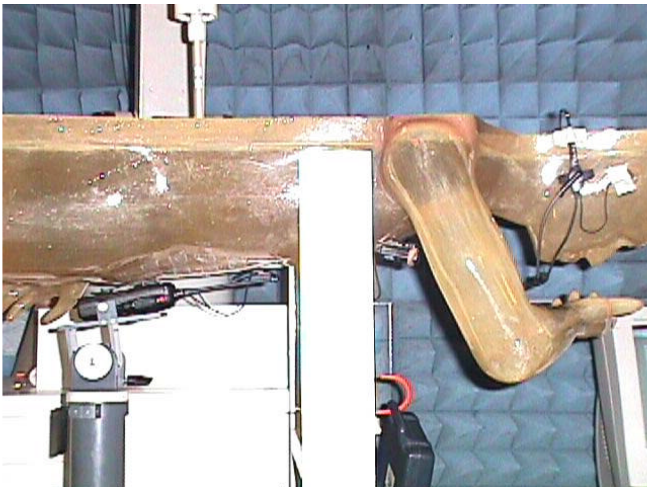
< Overview – Waist with the antenna positioned parallel to the phantom and the headset >
