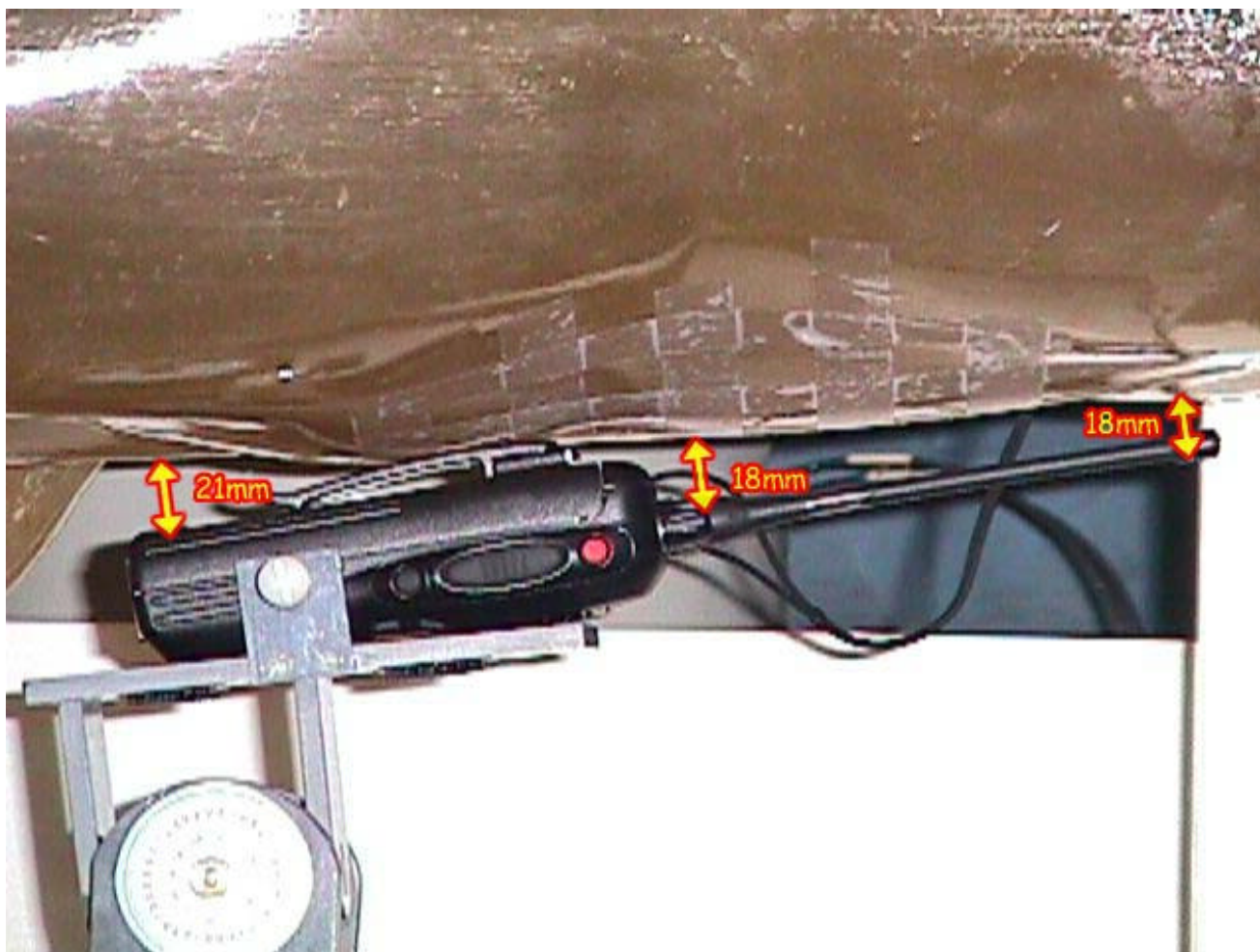
< Close-up view – Waist with the antenna positioned parallel to the phantom and headset>
