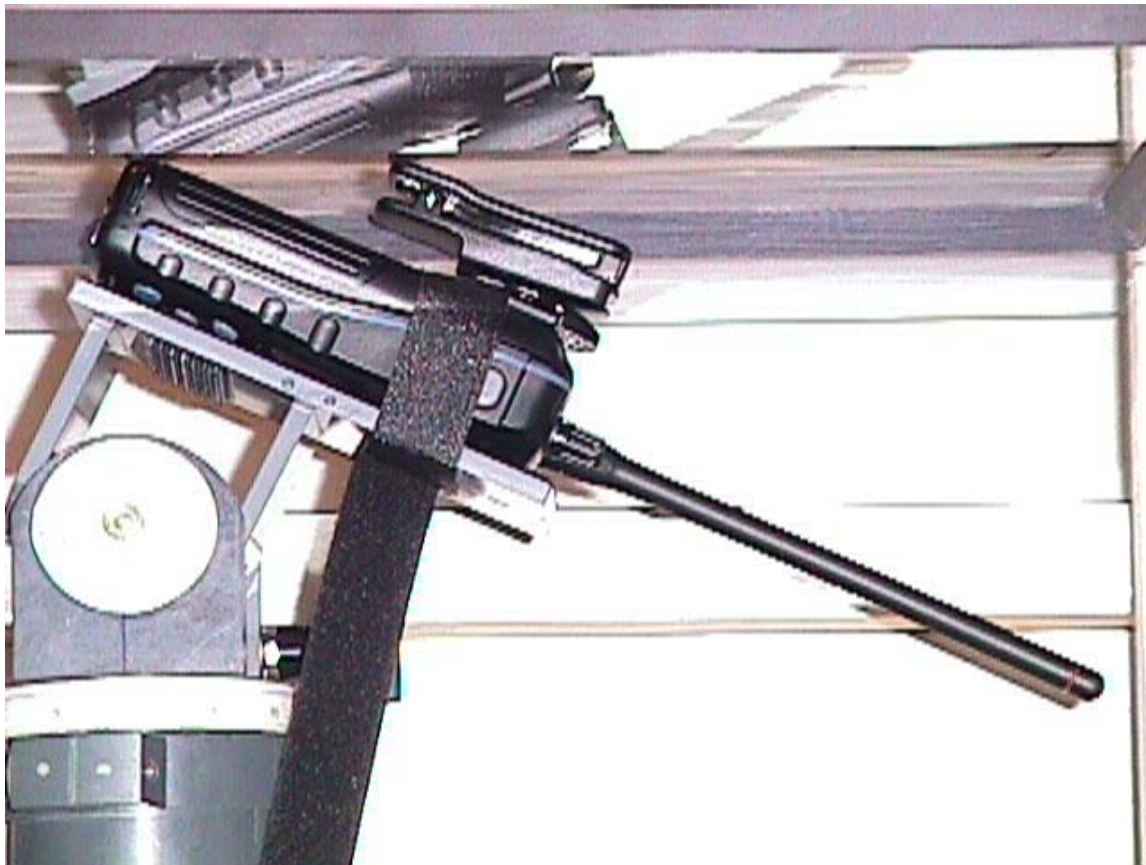
< The bottom of the EUT in contact with the phantom with the rotary belt clip(M/N: MB-87) – Overview >
