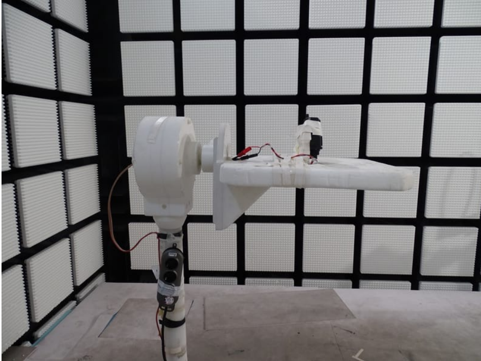
Photo 1: RSE setup 9 kHz to 30 MHz and > 1 GHz
