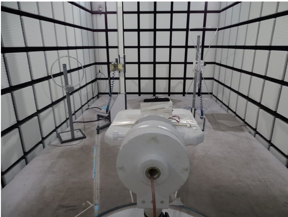
Photo 2: RSE setup 9 kHz to 30 MHz and > 1 GHz
