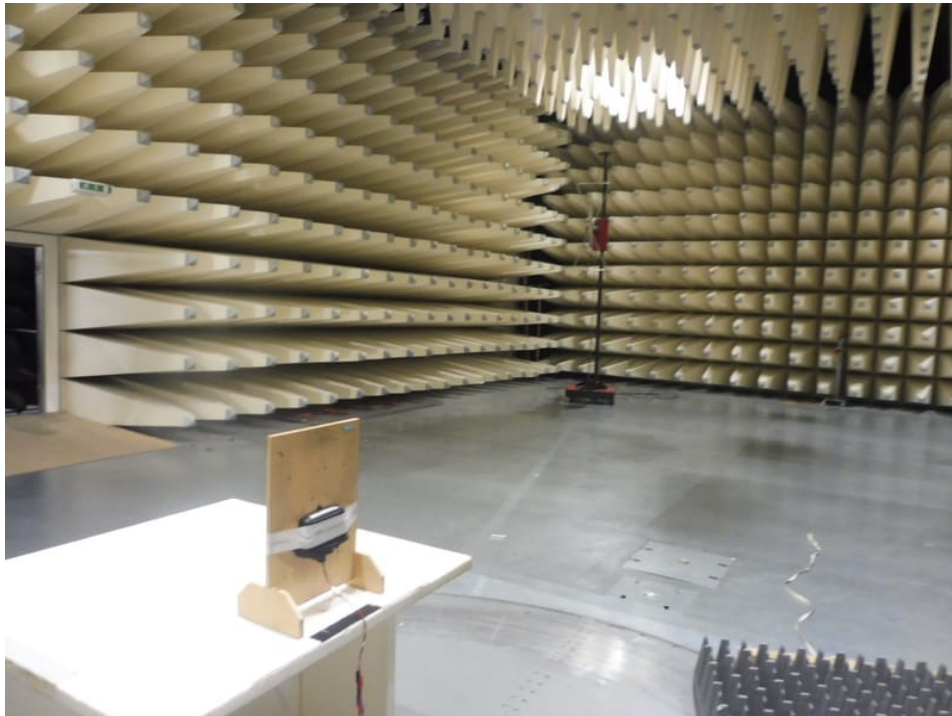
Photo 7: RSE setup 30 MHz to 1 GHz
