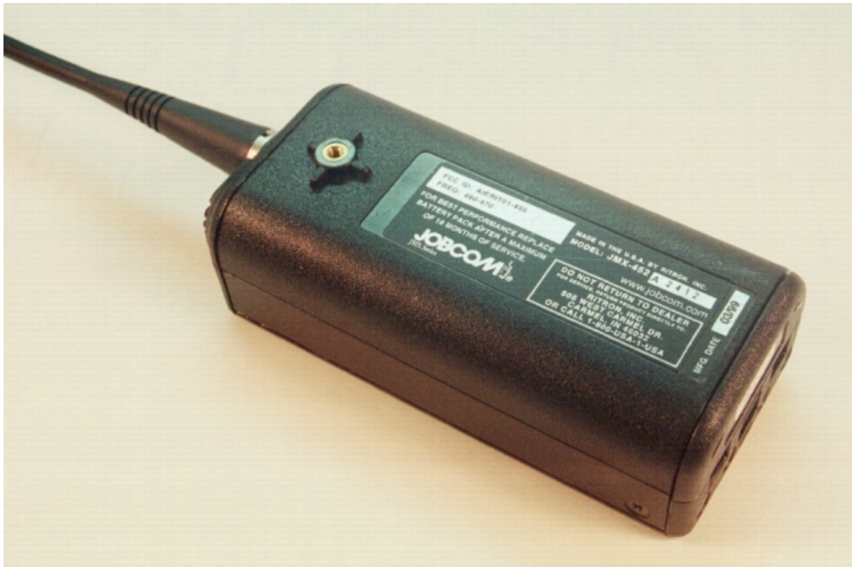
AIERIT13-442 SST-442 case back showing location of FCC identification label
