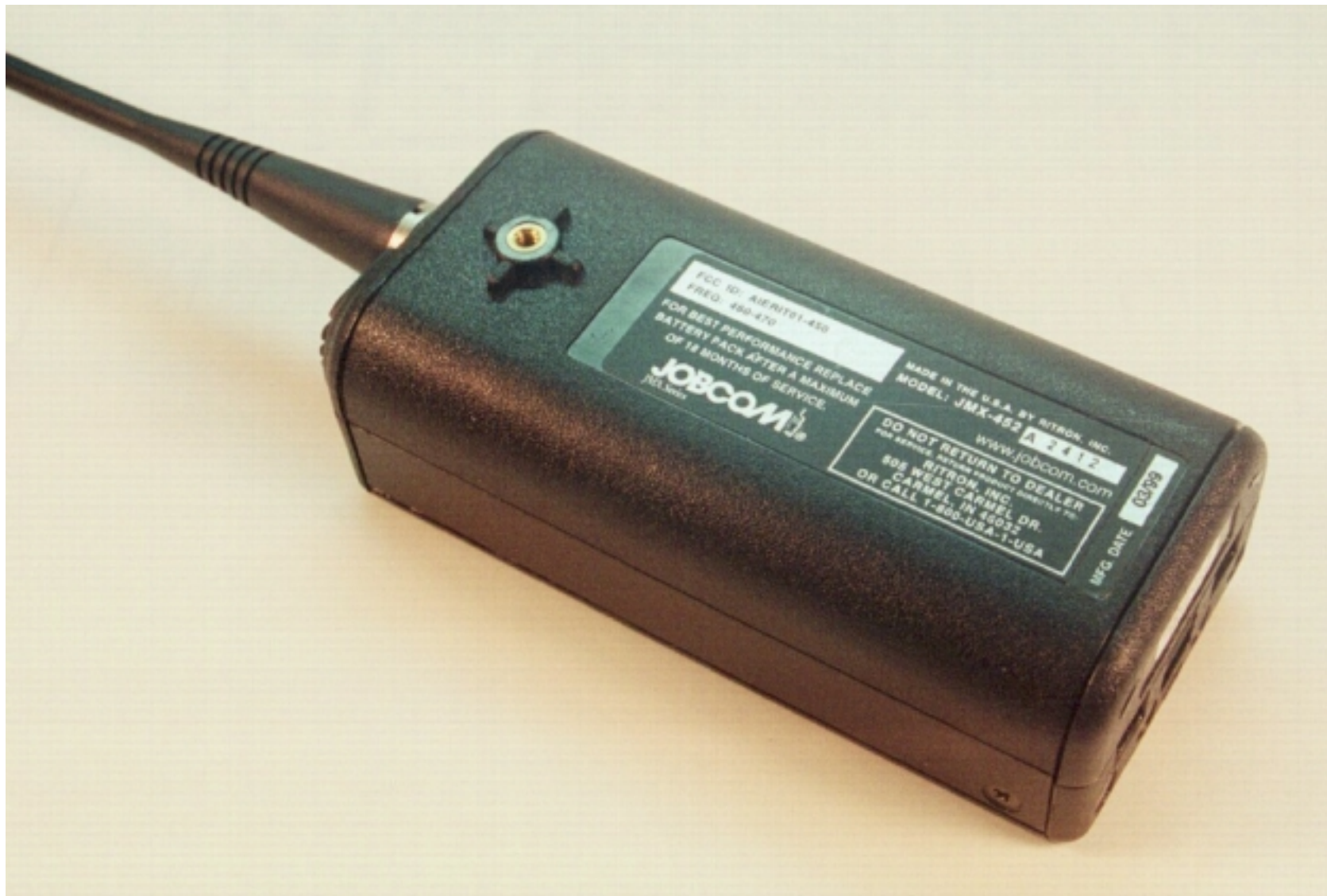
AIERIT13-450 SST-444 case back showing area for FCC identification label and belt clip installation
