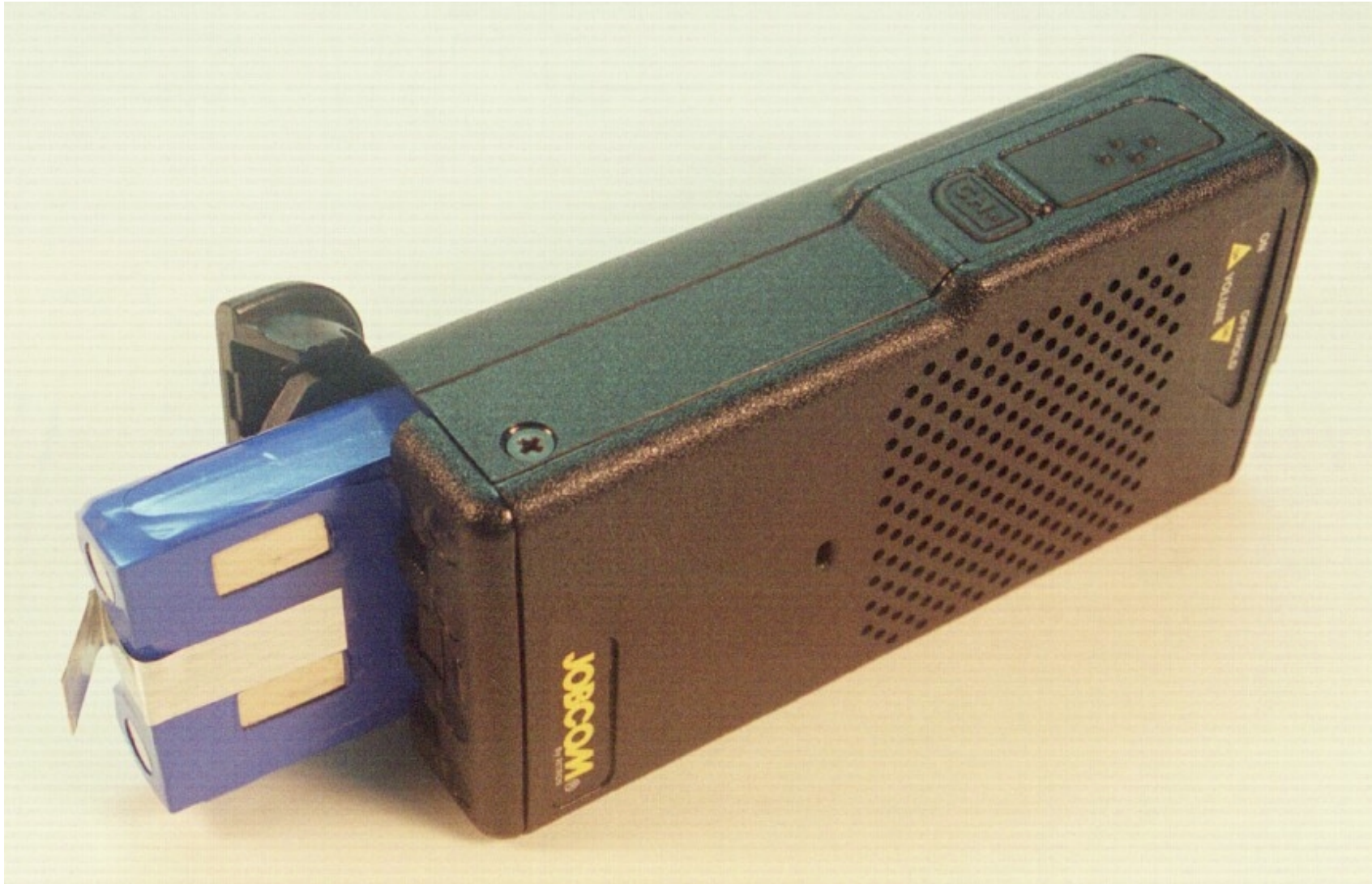
AIERIT13-450 SST-444 battery pack installation into case. PCB assembly, case bottom and battery insulator must be installed.
