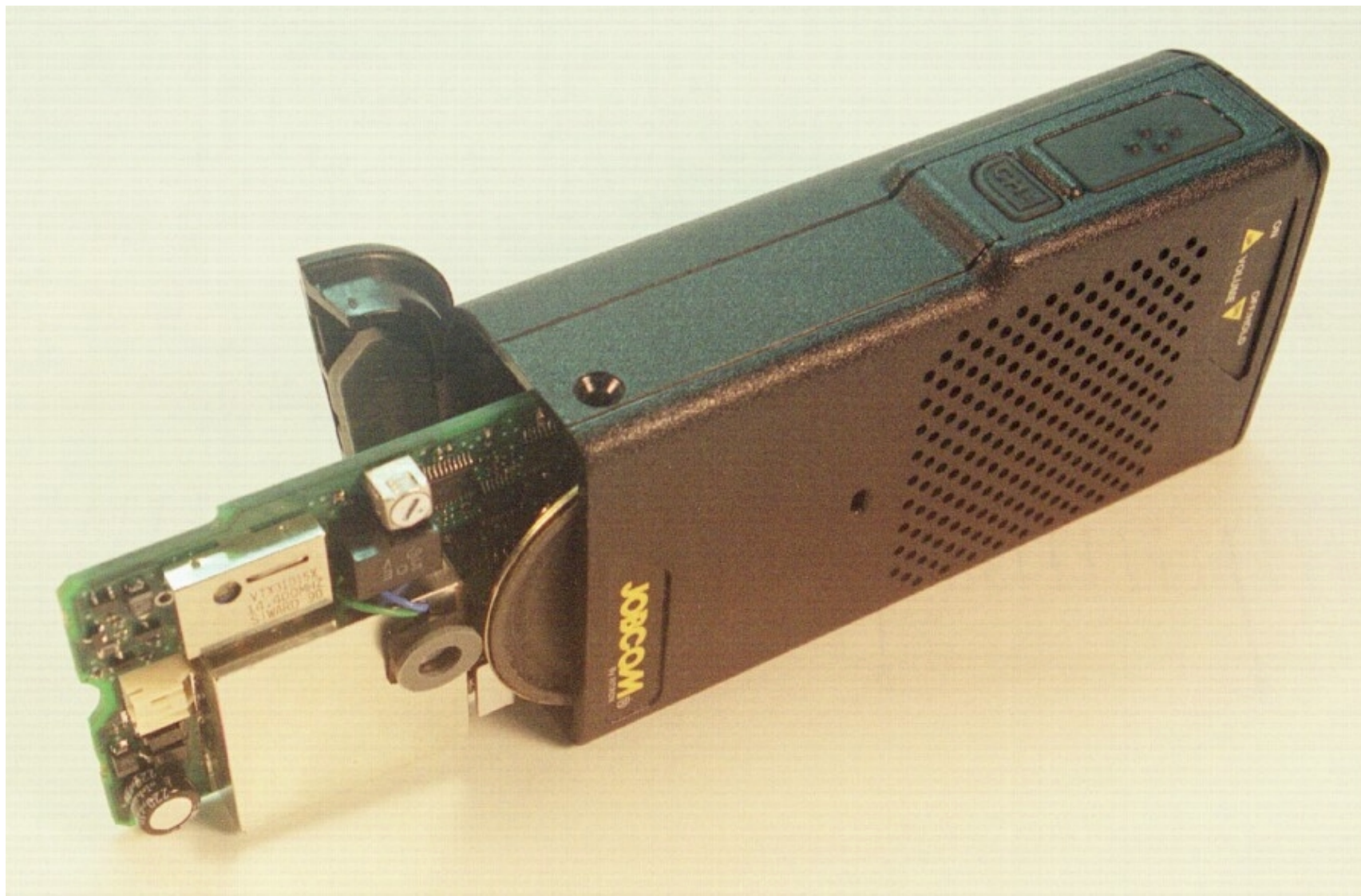
AIERIT13-450 SST-444 PCB installation into case.
