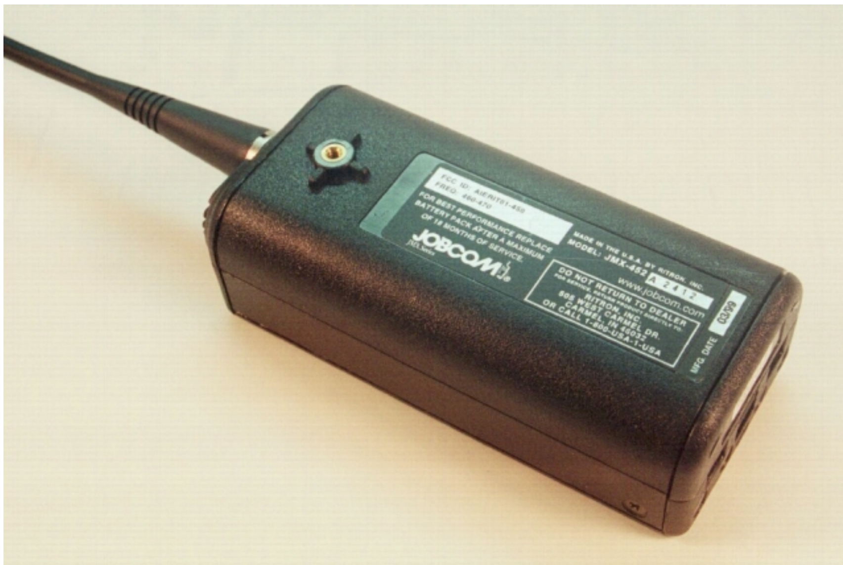
AIERIT13-450 SST-444 case back showing location of FCC identification label
