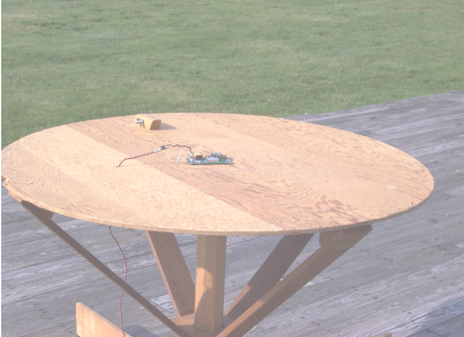
DR-442 on RITRON's 3 meter antenna range turntable
