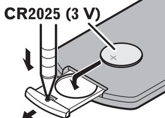
Insert the CR2025 (3 V) battery with the plus (+) and minus (-) poles orientated properly.
