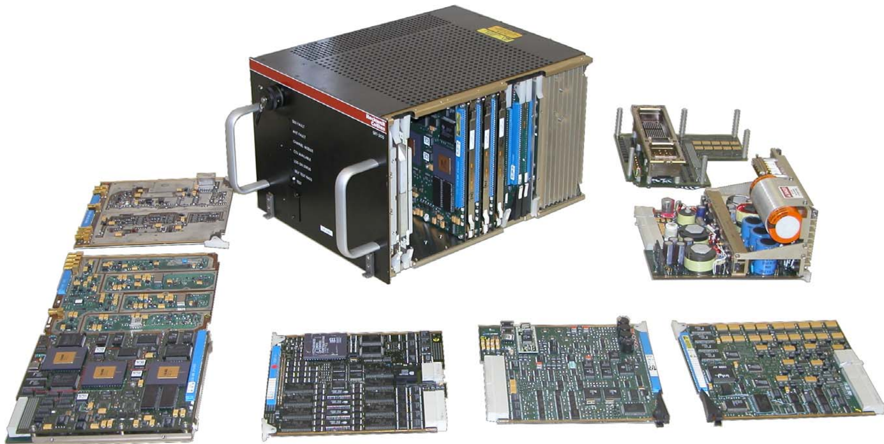
Figure 7-3. SRT-2100 Complement of Card Assemblies
