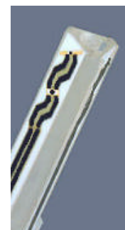
Figure 3.2 Probe Thick-Film Technique
