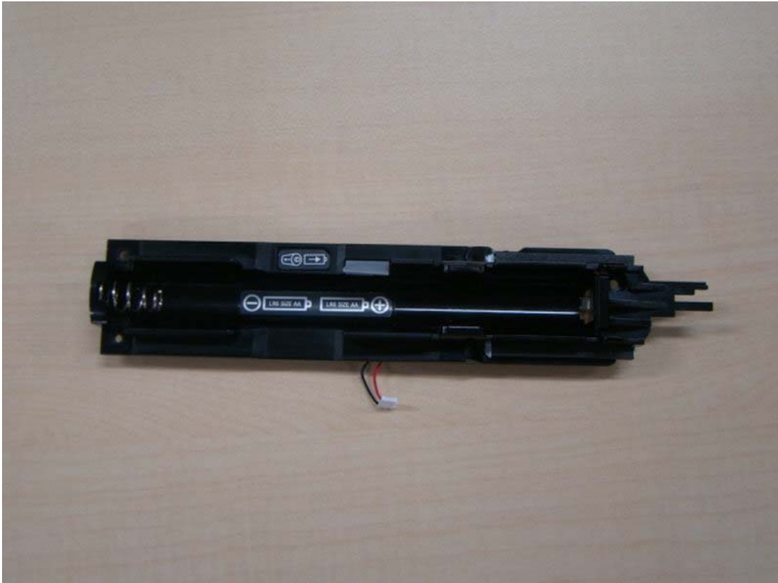
Fig.13: Rear side of the Battery case
