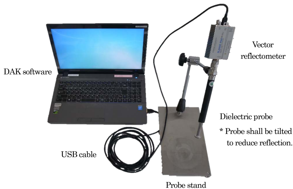
(a) Dielectric Parameter Measurement System
