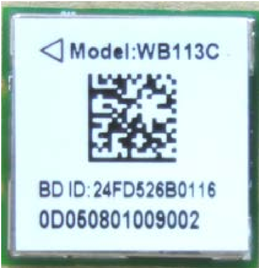
BLUETOOTH module: Top side with shield case
