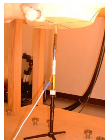
2450MHz System performance check setup
