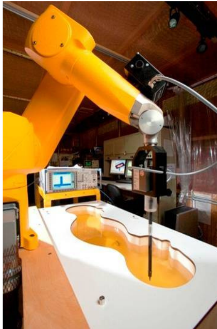
Figure 3-2 SAR Measurement System
