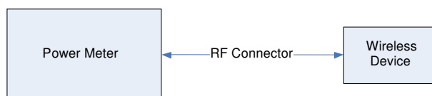
Figure 10-1 Power Measurement Setup
