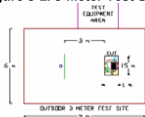
Figure 3-2. Dimensions of Outdoor Test Site
