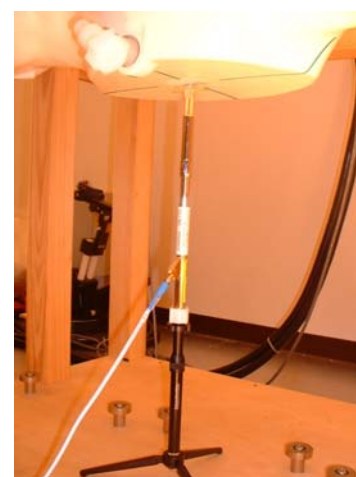
2450MHz System performance check setup
