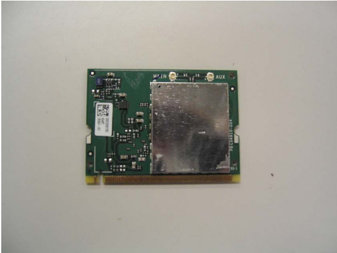
WLAN module: Side A with shield
