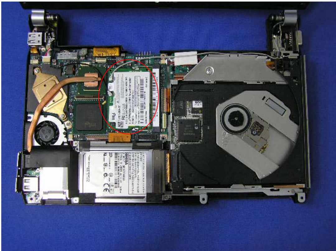
Location of WLAN module [Enlarged]
