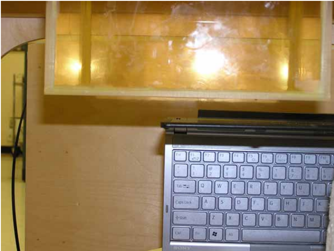
Photo 5: WLAN rear bystander main antenna
