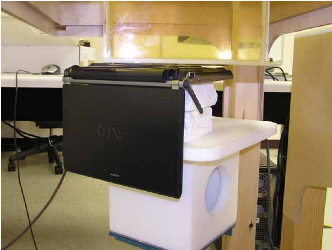
Photo 3: CDMA lap position antenna 45 degrees
