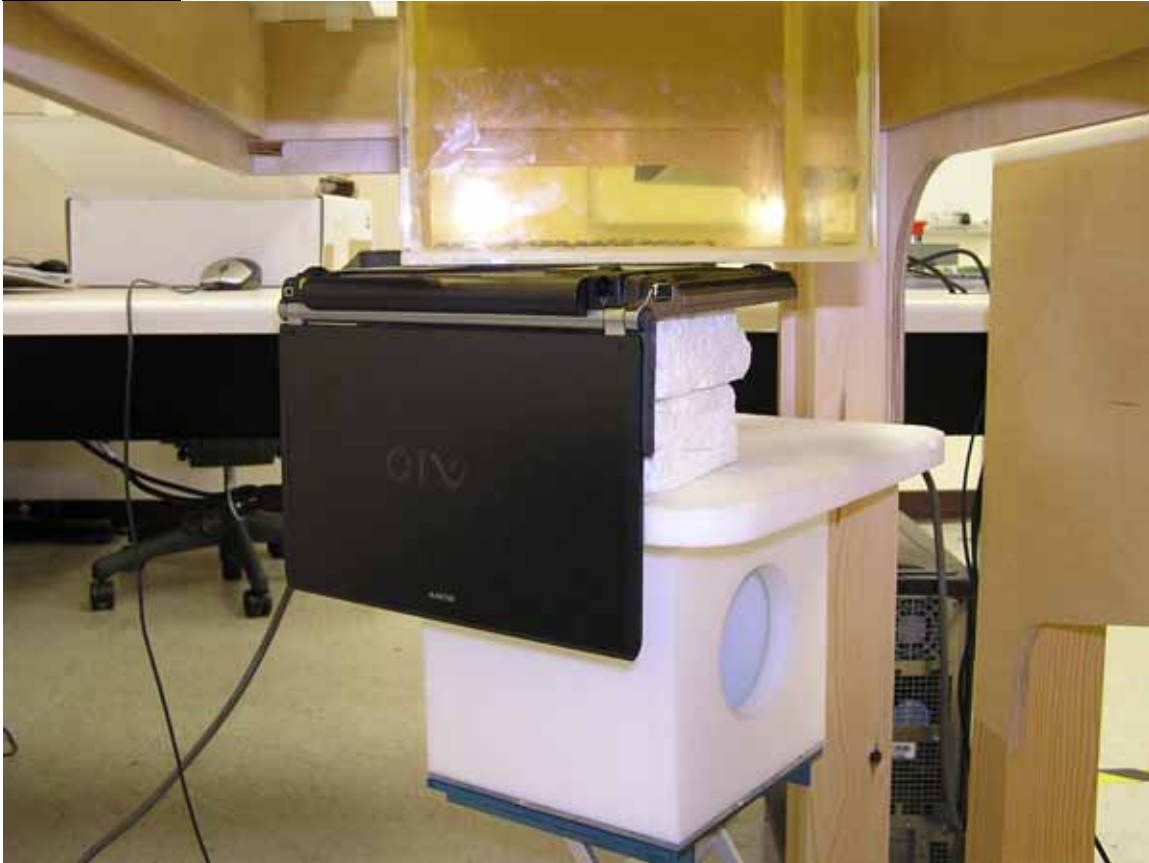
Photo 1: CDMA lap position antenna vertical
