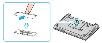
Align the bottom connector of the computer with the connector on the port replicator and push down until it clicks into place.
