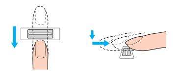
Keep your finger in contact with the fingerprint sensor while swiping.
