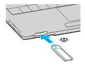
Be sure to hold the Memory Stick media with the arrow pointing in the correct direction as you insert it into the slot. To avoid damaging your computer or the Memory Stick media, do not force the Memory Stick media into the slot if you cannot insert it smoothly.
