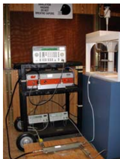
Figure 12.1 Dipole Validation Test Setup
