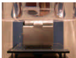
Figure 14.3.1 Body SAR Edge Normal Test Setup
