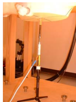
2450MHz System performance check setup
