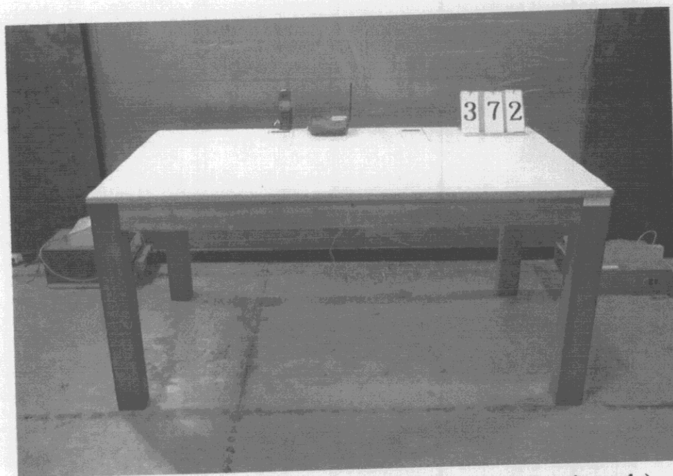
Fig. 2 Conducted emissions test placement (operating only)
