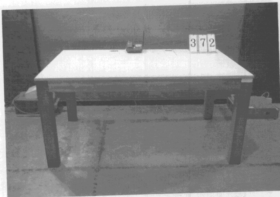
Fig. 1 Conducted emissions test placement (idle only)
