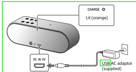
Charging starts when the unit is connected to an AC outlet via the **USB AC adaptor**, and the **CHARGE** indicator lights up orange. Charging is completed in about five hours and the indicator goes off.**How to Make Wireless Connection with BLUETOOTH Devices**
