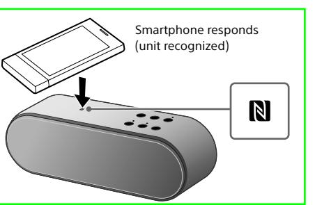
Follow the on-screen instructions to establish the connection. When the BLUETOOTH connection is established, the Ø (BLUETOOTH) indicator on the unit stays lit. To disconnect, touch the unit with the smartphone again.
