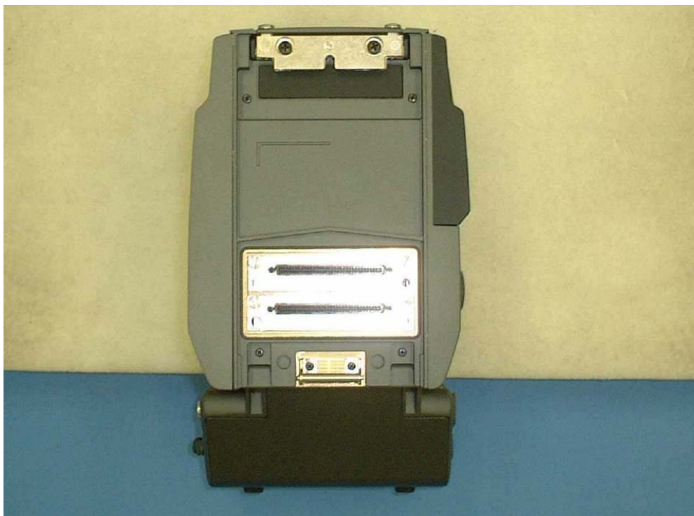
Rear View of Wireless Transmitter
