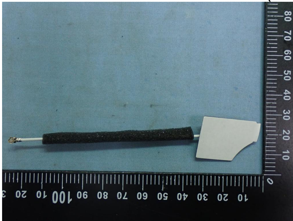
Figure 33 Antenna of the EUT (ZTX-RH5- BT-V02)
