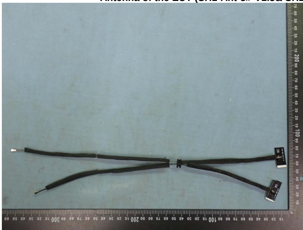
Figure 13 Antenna of the EUT (SH1-Ant-3#-V1.3& SH1-Ant-4#-V1.3)
