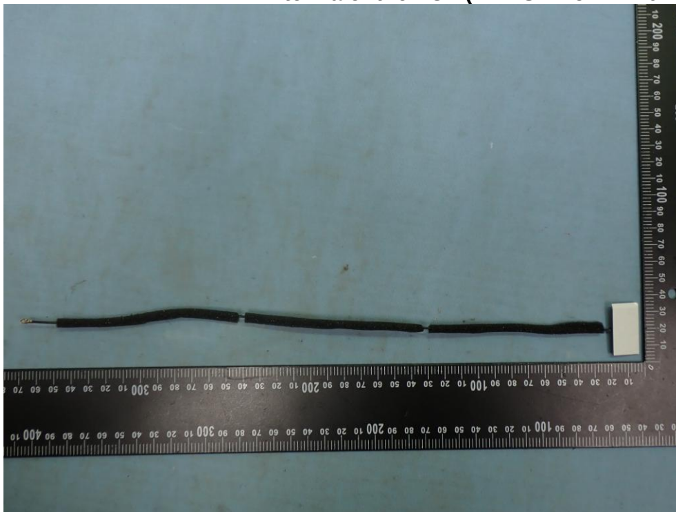
Figure 52 Antenna of the EUT (ZTX-SWH5-WIFI-0-V02 (WIFI0))
