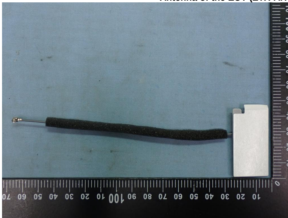
Figure 24 Antenna of the EUT (ZTX-AHC-BT -V03 )
