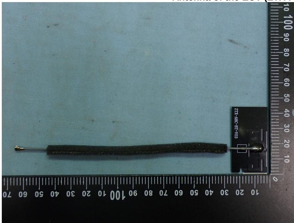
Figure 23 Antenna of the EUT (ZTX-AHC-BT -V03 )
