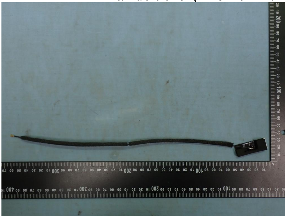
Figure 41 Antenna of the EUT (ZTX-SWH3-WIFI-0-V04 (WIFI0) )
