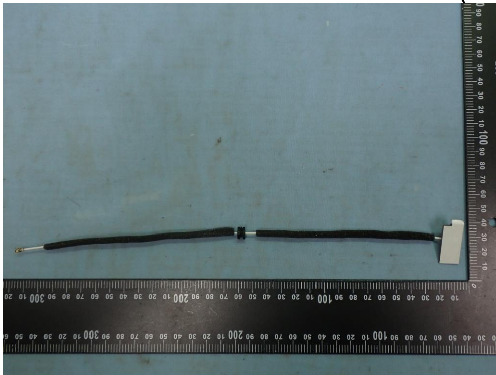
Figure 11 Antenna of the EUT (SH1-Ant-5#-V1.3)
