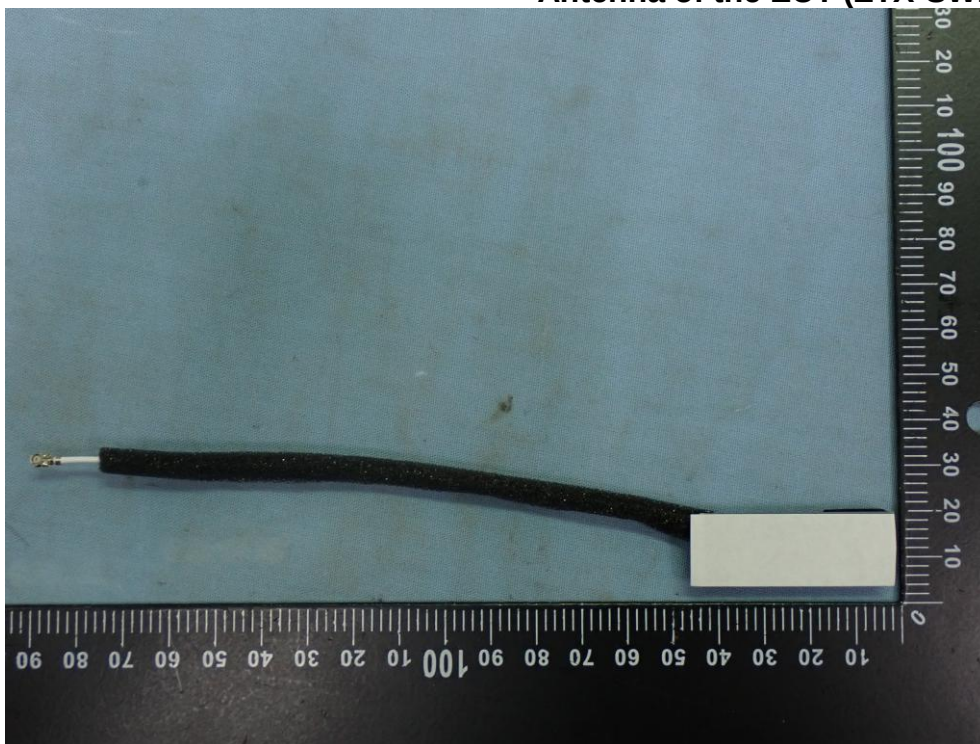
Figure 48 Antenna of the EUT (ZTX-SWH3-BT-V04)
