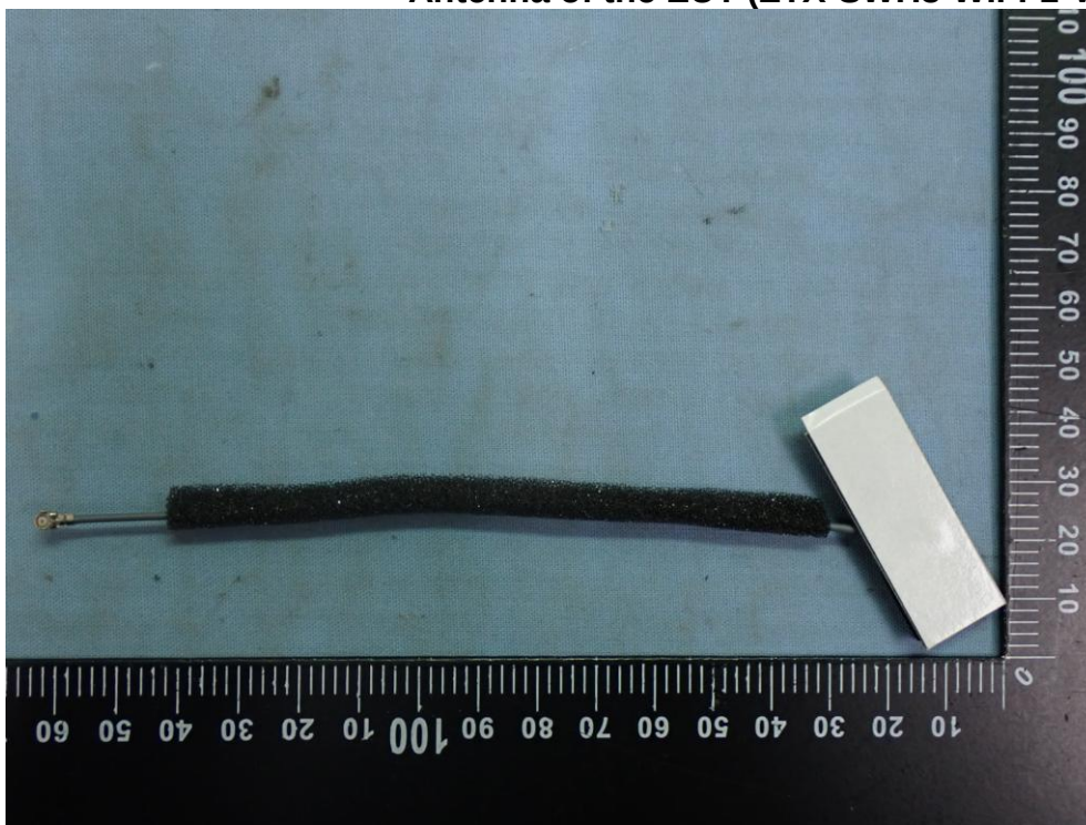
Figure 45 Antenna of the EUT (ZTX-SWH3-WIFI-1-V02 (WIFI4))
