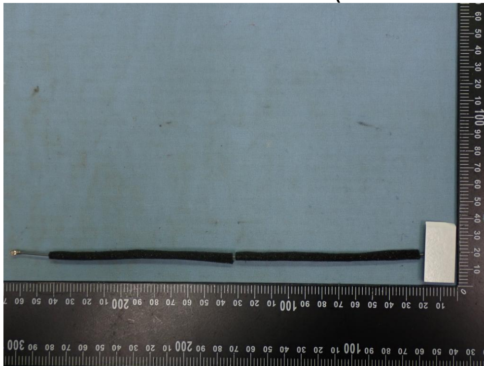
Figure 39 Antenna of the EUT (ZTX-AHS- Ant-3#-V02 (WIFI0) )
