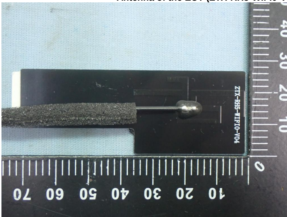
Figure 28 Antenna of the EUT (ZTX-RH5-WIFI0-V04 (WIFI0) )
