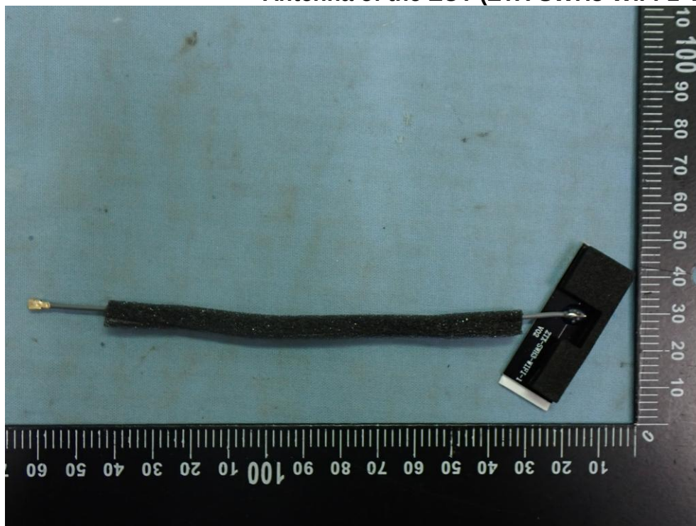
Figure 44 Antenna of the EUT (ZTX-SWH3-WIFI-1-V02 (WIFI4))
