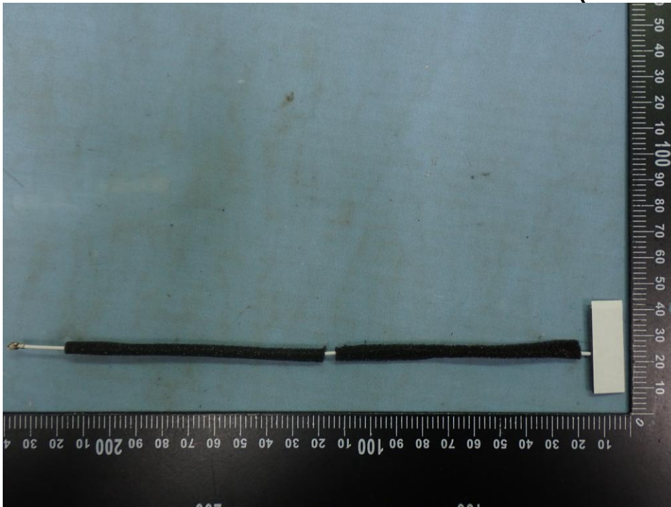
Figure 58 Antenna of the EUT (ZTX-SWH5-BT-V01)
