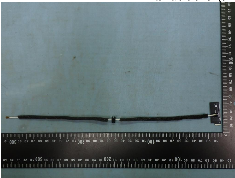
Figure 10 Antenna of the EUT (SH1-Ant-5#-V1.3)
