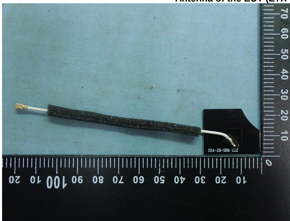
Figure 32 Antenna of the EUT (ZTX-RH5- BT-V02)
