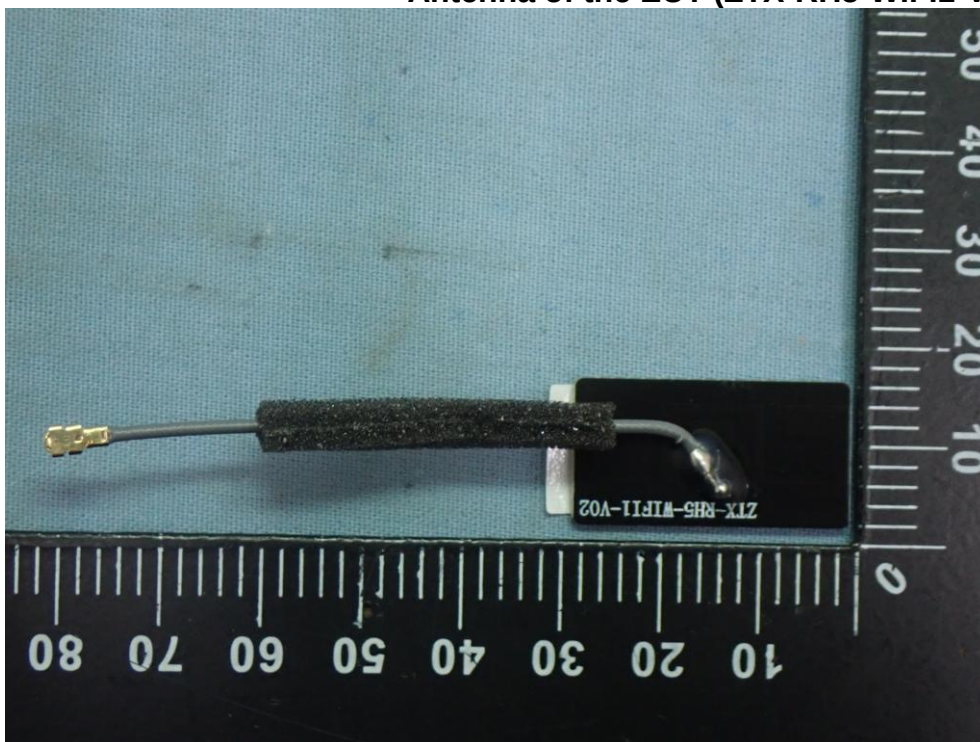
Figure 29 Antenna of the EUT (ZTX-RH5-WIFI1-V02 (WIFI1))
