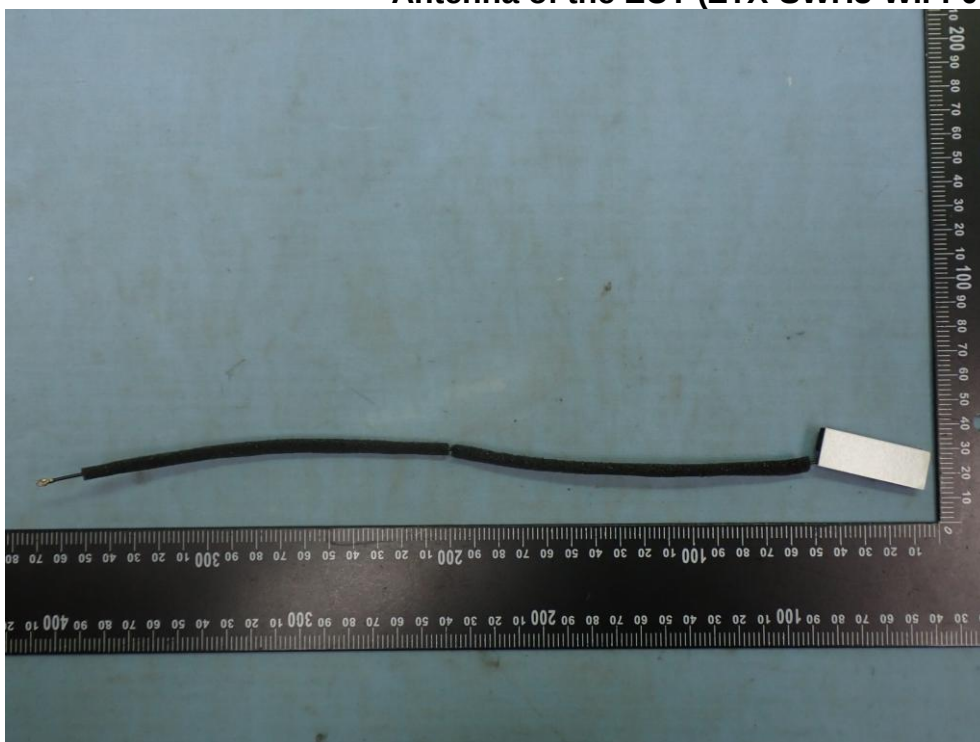
Figure 42 Antenna of the EUT (ZTX-SWH3-WIFI-0-V04 (WIFI0) )
