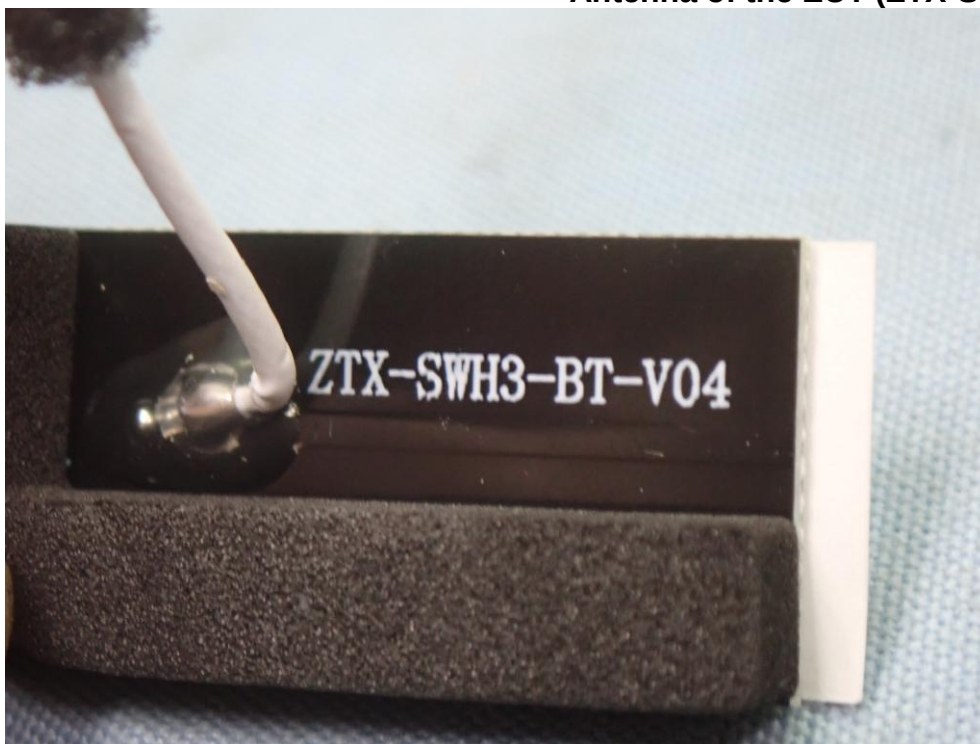
Figure 50 Antenna of the EUT (ZTX-SWH3-BT-V04)
