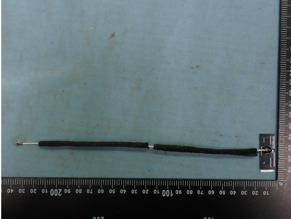
Figure 57 Antenna of the EUT (ZTX-SWH5-BT-V01 )
