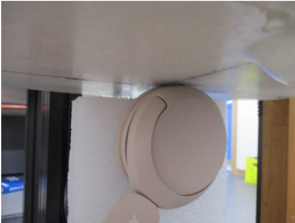
Antenna Touching - Left Side from Flat Phantom (Separation Distance: 0 cm)
