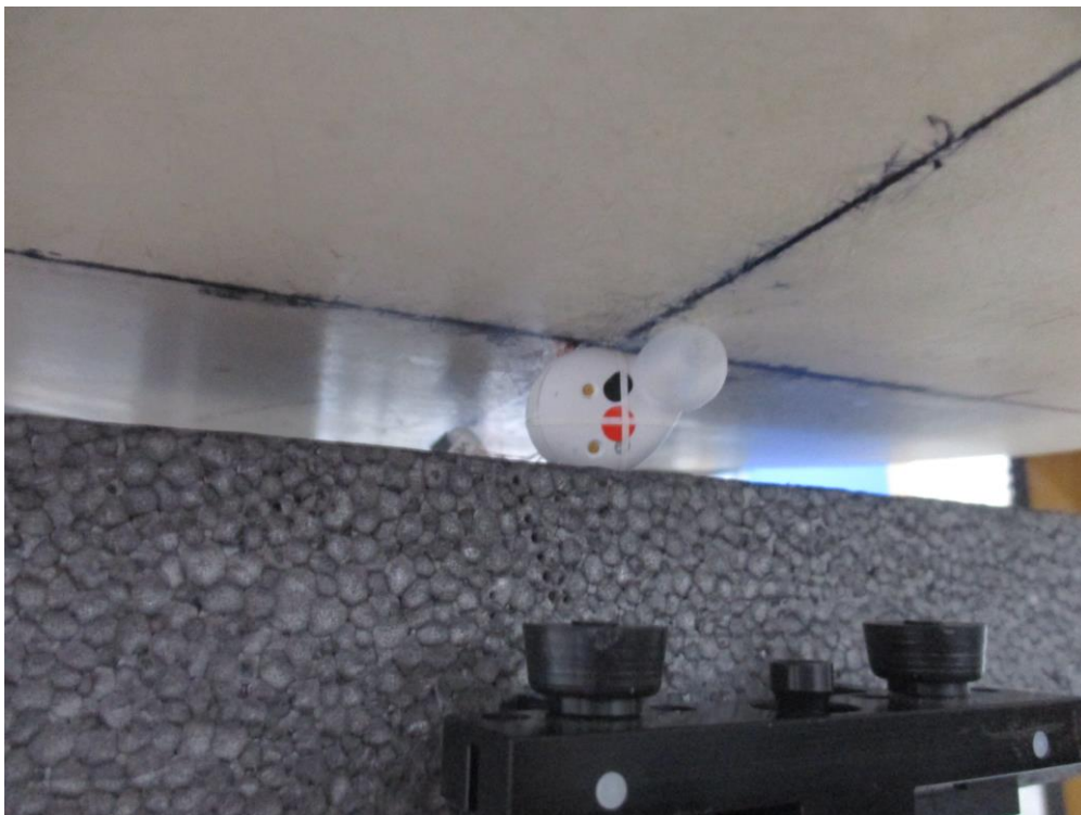
Left Side from Flat Phantom (Separation Distance: 0 cm) – Left Ear
