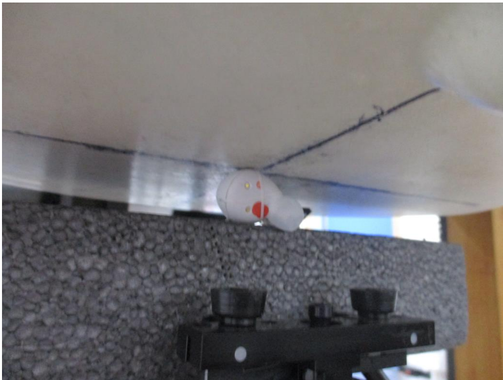
Left Side from Flat Phantom (Separation Distance: 0 cm) – Right Ear
