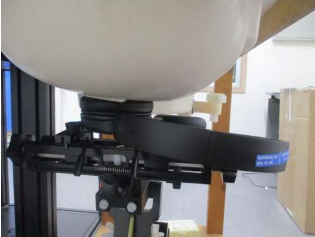
Right Head from SAM Twin Phantom (Separation Distance: 0 cm)
