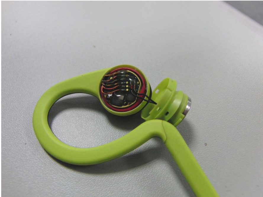
Left PCBA Installed
