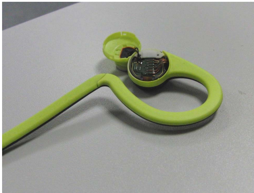
Right PCBA Installed
