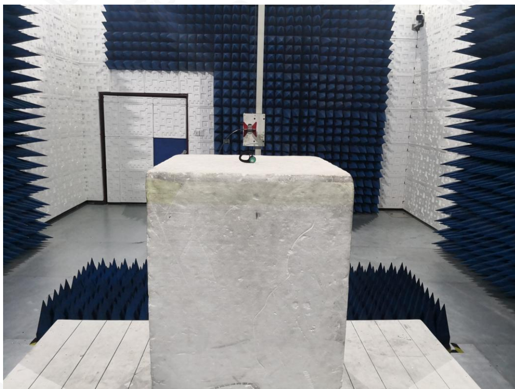
RADIATED EMISSION TEST SETUP ABOVE 1GHZ
