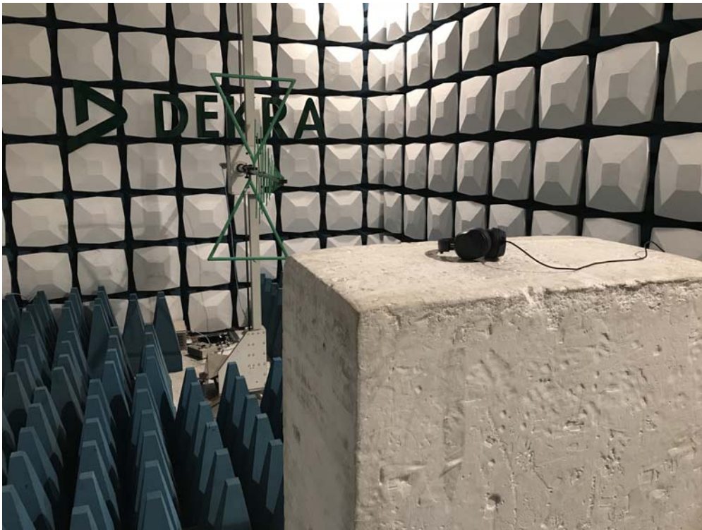
Description: Radiated Emission Test Setup for 1~18GHz
