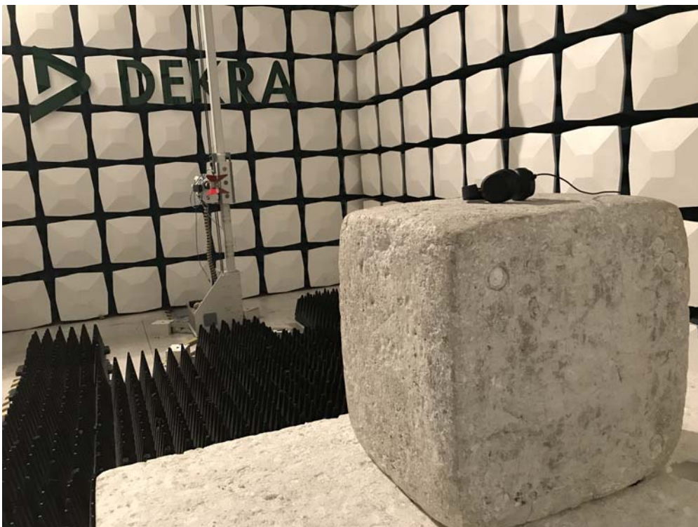
Description: Radiated Emission Test Setup for 1~18GHz
