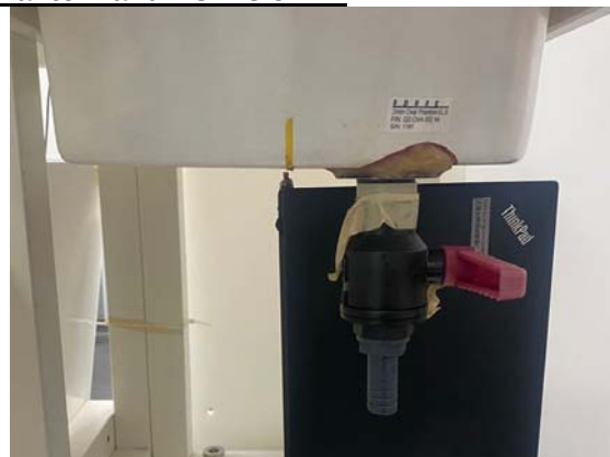
Fig.6 EUT Tip_without cable side to flat phantom
