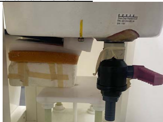
Fig.3 EUT Horizontal-Down side to flat phantom
