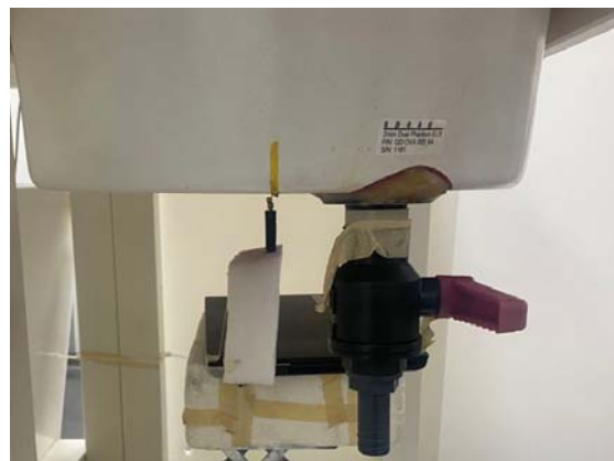
Fig.5 EUT Tip_with cable side to flat phantom
