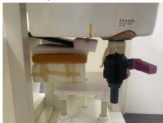
Fig.7 EUT Vertical-Back side to flat phantom
