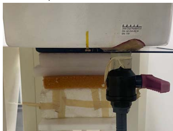
Fig.4 EUT Horizontal-Up side to flat phantom
