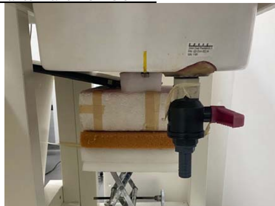
Fig.3 EUT Horizontal-Down side to flat phantom
