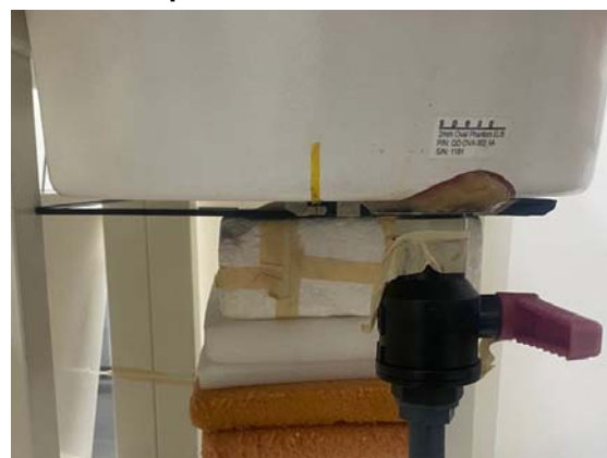
Fig.4 EUT Horizontal-Up side to flat phantom
