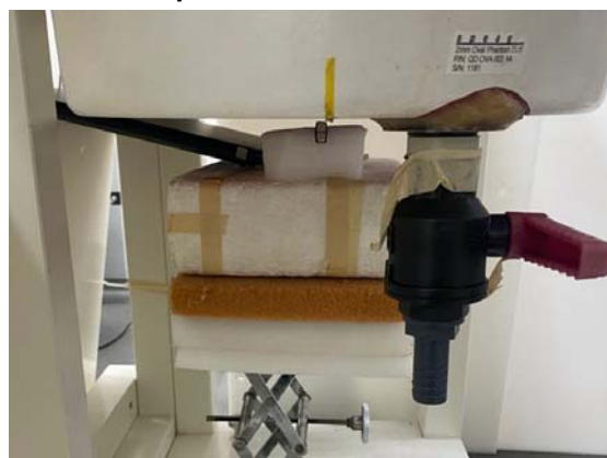
Fig.7 EUT Vertical-Back side to flat phantom
