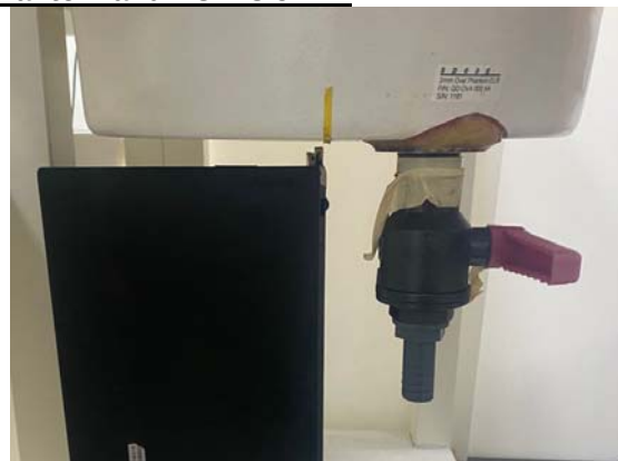
Fig.6 EUT Tip _without cable side to flat phantom
