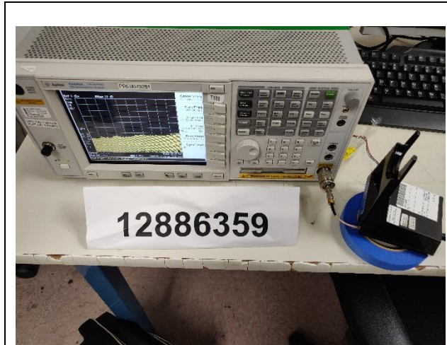
RF ANTENNA PORT CONDUCTED
