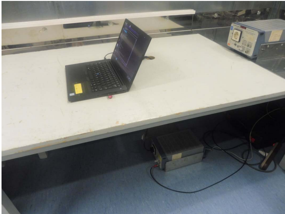
Photo 1: Conducted Emission Test
