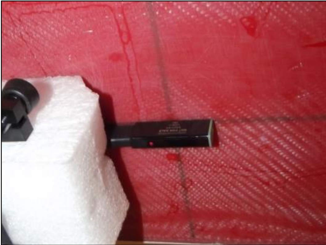
Photo 10: Test position - Right side with 0mm distance
