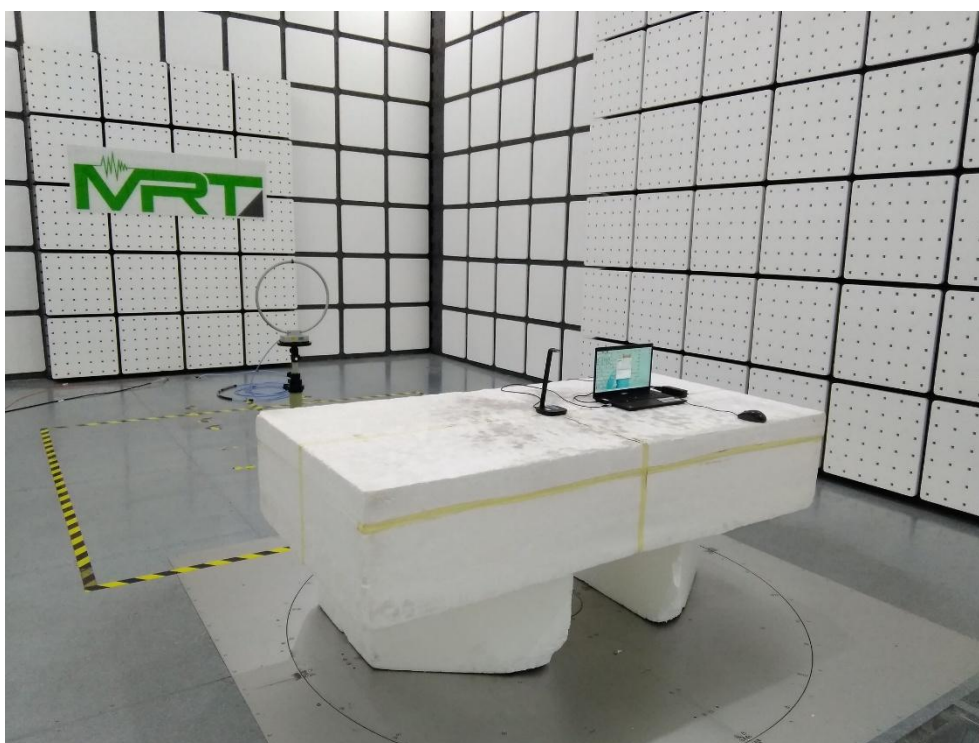
Description: Radiated Emission Test Setup for 9kHz~30MHz
