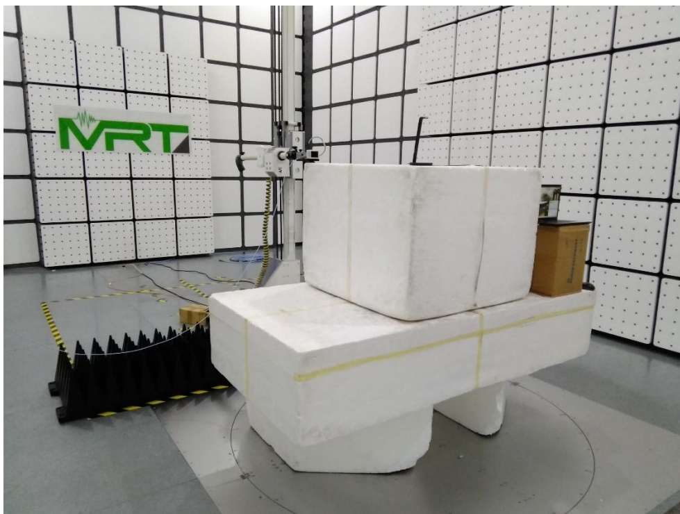
Description: Radiated Emission Test Setup for 9kHz~30MHz
