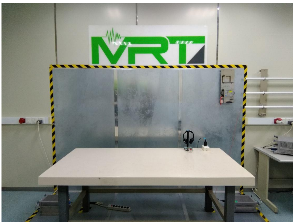
Description: Back View of Conducted Emission Test Setup _Mode 4
