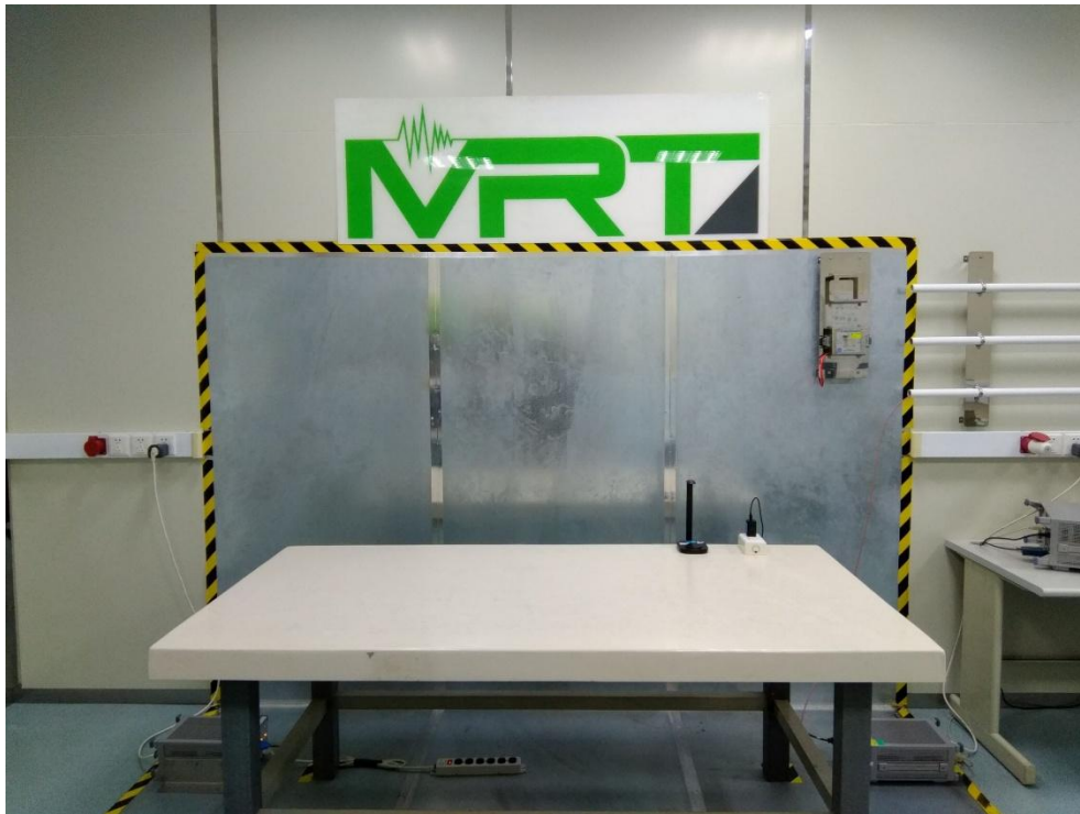
Description: Back View of Conducted Emission Test Setup _Mode 6
