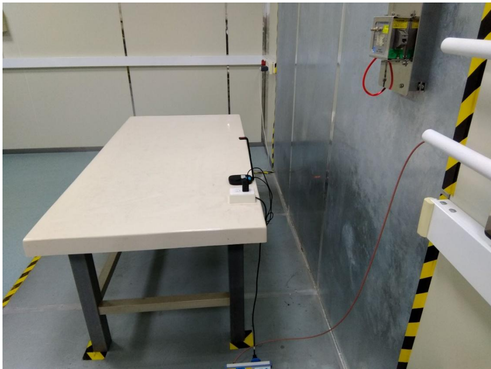
Description: Back View of Conducted Emission Test Setup _Mode 6
