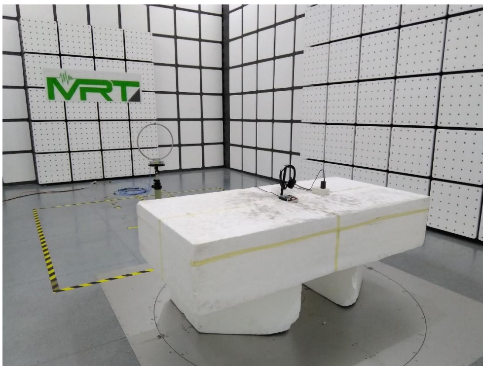
Description: Radiated Emission Test Setup for above 30MHz_Mode 2
