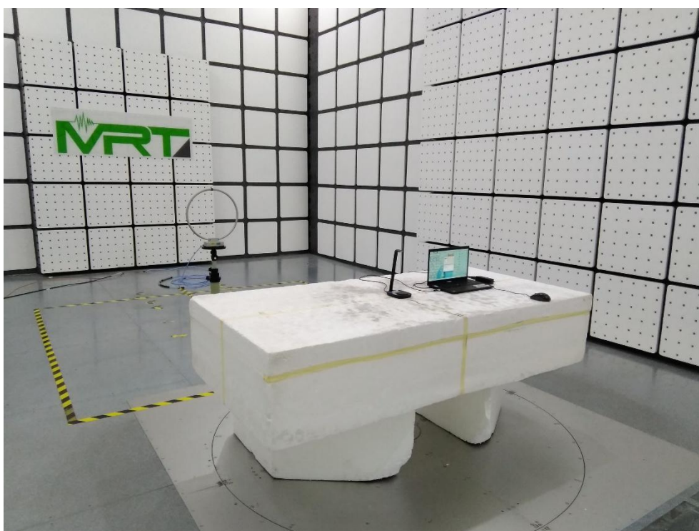
Description: Radiated Emission Test Setup for 9kHz~30MHz
