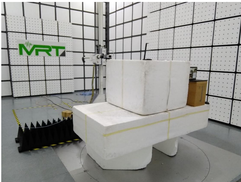
Description: Radiated Emission Test Setup for 9kHz~30MHz
