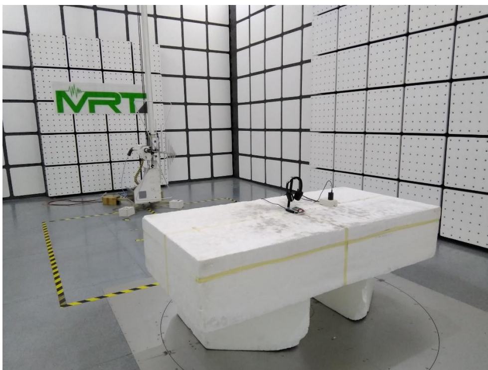
Description: Radiated Emission Test Setup for above 30MHz_Mode 2
