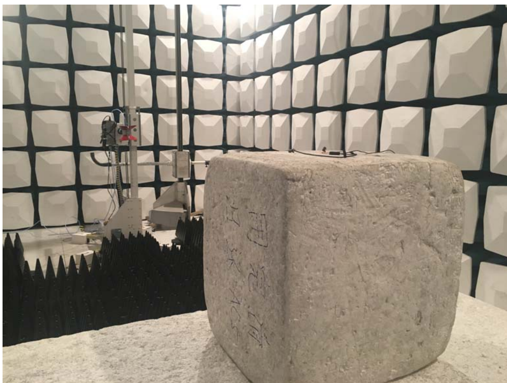
Description: Radiated Emission Test Setup for 1~18GHz
