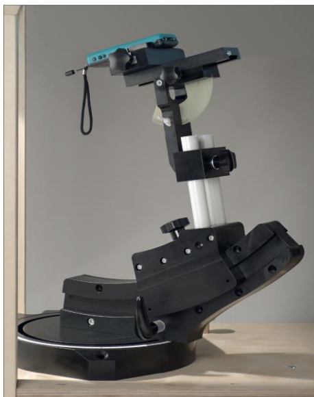
F-2. Device Holder for Transmitters
