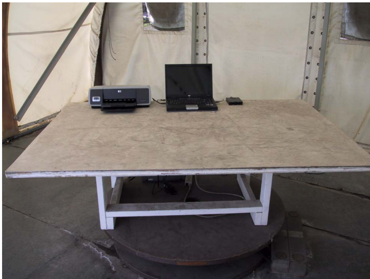
Radiated Emissions Test Setup – Front
