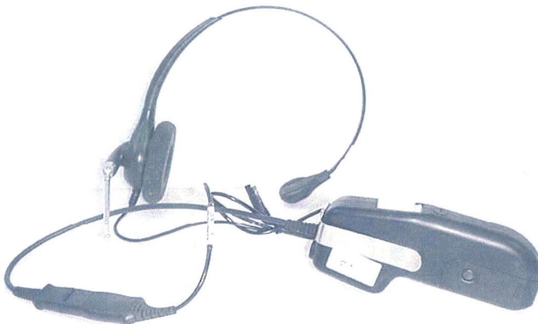
Remote Unit with Plantronics SupraPlus Headset (H251)
