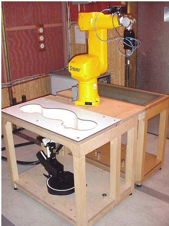
DASY4 SAR Measurement System with SAM Phantom
