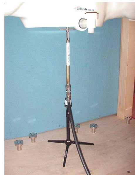
1900MHz Dipole Setup
