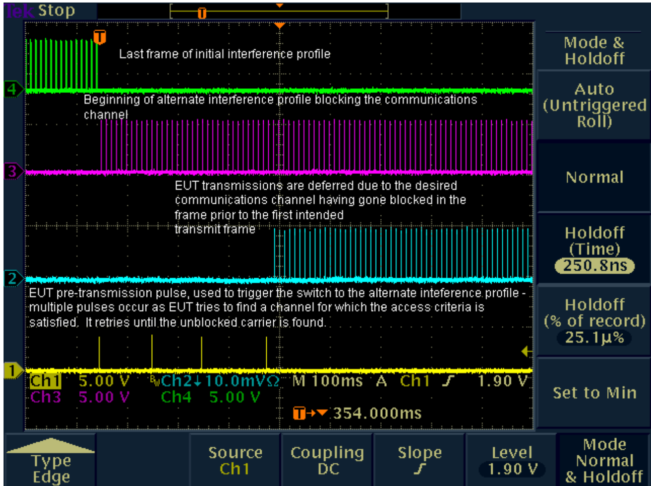
Fig. 50 - Screen shot of oscilloscope showing deferral by the headset EUT in the case where the interference profile changes in the frame previous to intended transmission and the selected time and frequency communications channel becomes blocked; and then later, transmission on unblocked channel.
